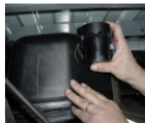
Figure C3, Step 3: Slide fuel valve from bracket.
